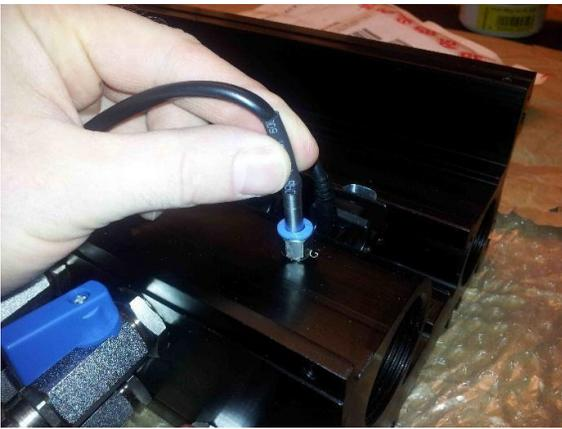
5. Push the temperature sensor into the blue fitting, and try to pull it to secure that it is fastened.
