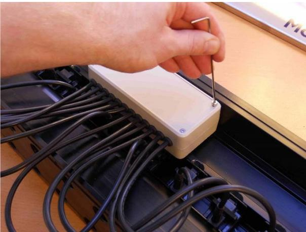
2. Refit the 2 M3x45 countersunk mounting screws.
