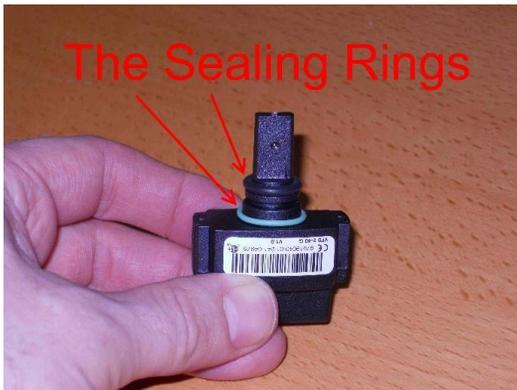
1. Make sure that both sealing rings are on the new
