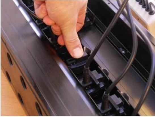
3. Then push down the sensor, so the sealing rings are sealed tight.
