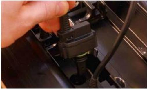
4. Remove sensor and make sure the 2 sealing rings (o-rings) are removed as well
