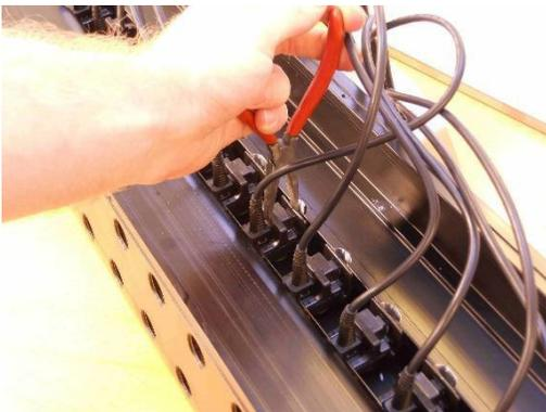
2. Release the metal clips manually or with a small plier.
