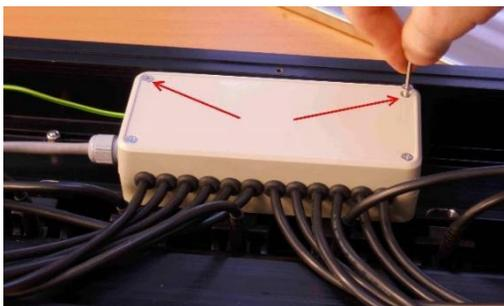
3. Remove the 2 Hex screws (M3x45 countersunk).
