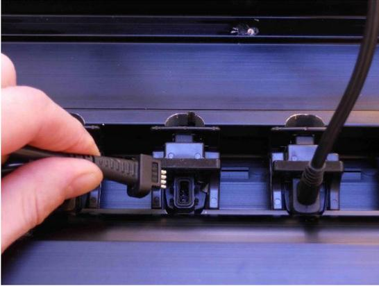
6. Gently connect the plug, be careful not to bend any of the sensor pins in the socket.
