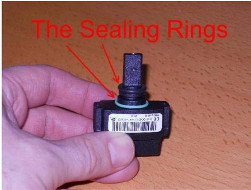
7. Make sure the sealing rings are not left in the sensor
