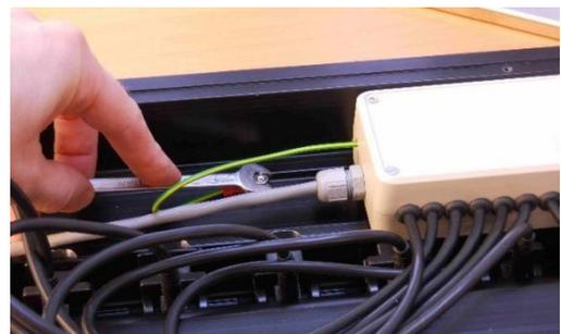
2. Remove the nut, holding the ground wire (M4).
