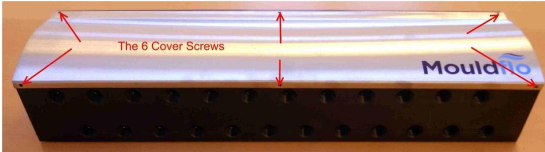
Remove the 6 cover screws. (M4x6) then lift off the cover.
