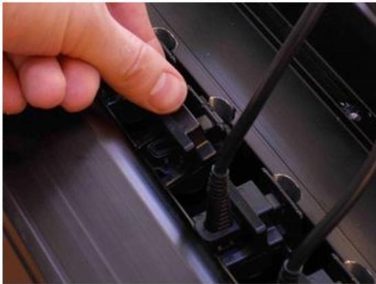
4. Place the clips over the sensor, so that the socket is accessible.
