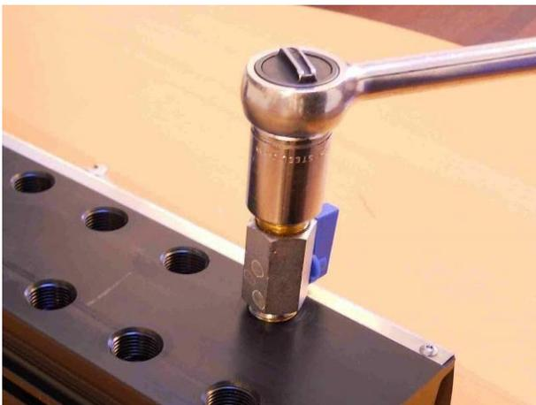
2. Tighten the valve so the valve handle is not in the way of the other valves.
